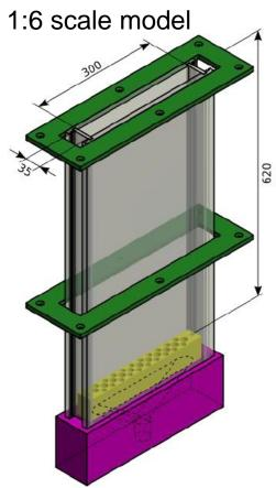
Stirring system with 6 coils (only traveling field setup)
