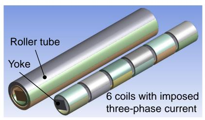
Ansys Emag: Electromagnetic field and forces are calculated (for a resting fluid) in a harmonic simulation at stirring frequency
