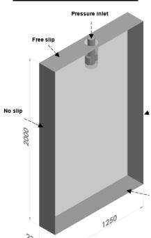
Casting speed: v<sub>in</sub>=1.0 m/min
