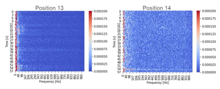
> However: the **influence of the position on the spectrum** is more noticeable, e.g. due to the water jet of the descaling system evaporating on the strand surface
