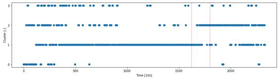
Conclusion from measured population of spectra classes to position of crater end in front of or behind the measurement position
